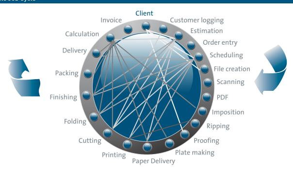
It's a long road from Estimate to Invoice, and keeping customer service people in the loop with up-to-the-minute info is easy when presses are equipped with JDF (Job Definition Format) and JMF (Job Message Format) links that communicate to a central MIS system.
