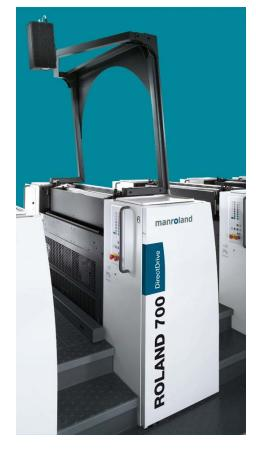
Can you spot a hickey at 15,000 sph? This camera can. Not only that, it can instantly alert the operator at the console and, if the press is equipped with a direct, programmable Delta dampener, he can simply press a button and fix the problem in seconds!
