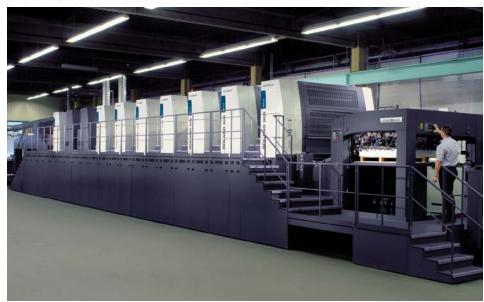
From computer controlled inking and color monitoring, to automated plate loading, blanket washing and more, today's large format presses deliver output quality along with makeready ease and speed equal to or better than mid-sized machines ... and put many more sheets on the floor at the end of the day.
