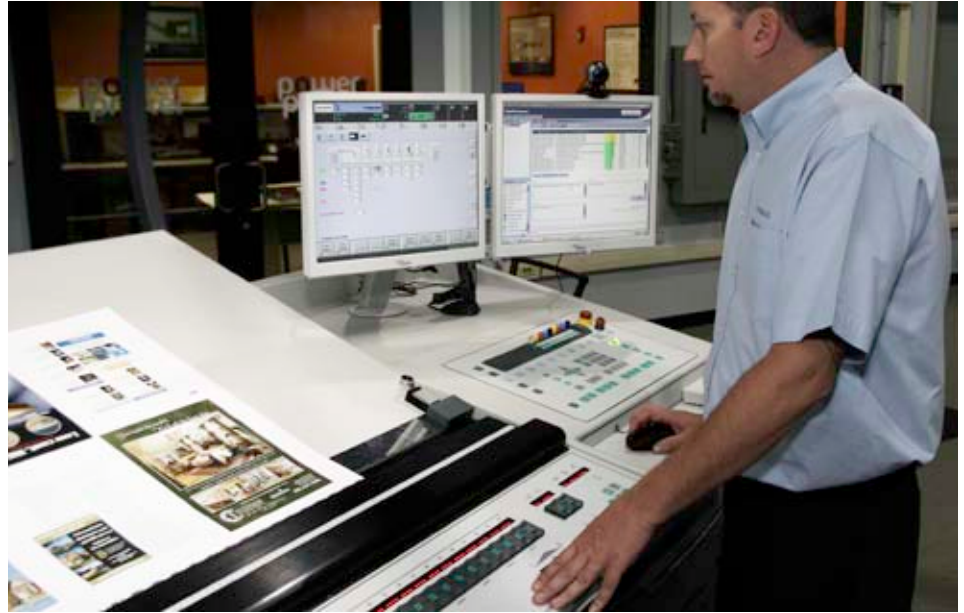
On-the-Fly Image Registration Adjustment: The latest-generation multitasking 40-inch presses enable the operator to adjust image length on-the-fly from the console in seconds, which saves downtime while also allowing you to maintain high-speed production with lighter weight stocks.
